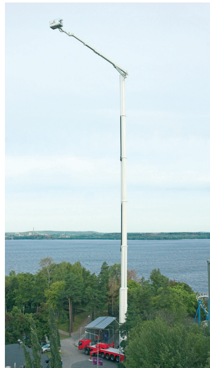
Fig. 5. F 101 HLA has the working outreach of 28 meters.
