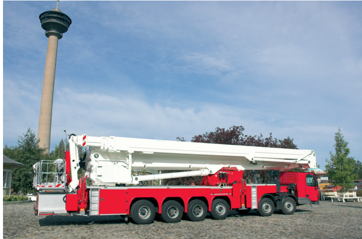
Fig. 3. The first 101 m has been built for the Belgian rental company Maes. The unit is mounted onto Mercedes Benz 6258 Actros 12X4 chassis.
